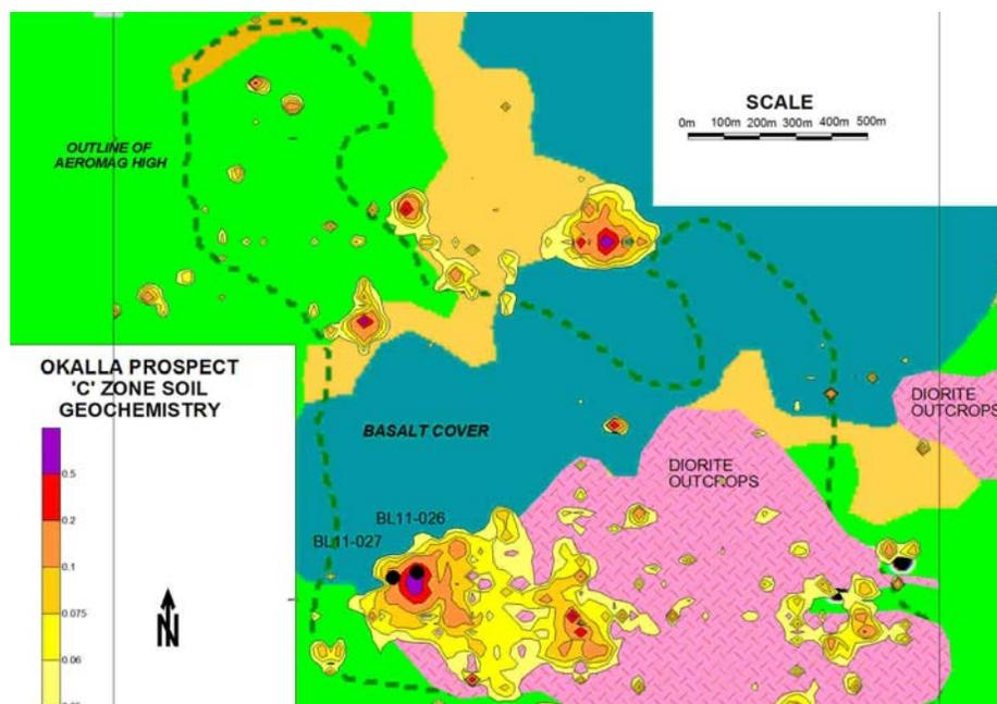
The geochemical anomaly terminates to the north against an overlying Quaternary flood basalt flow. An extension to the geochemical survey shows a further gold-copper soil anomaly about 1km to the northeast, beyond the basalt ridge. The accompanying map shows the location of these two holes in relation to the gold anomalies overlain on the simplified geology.
